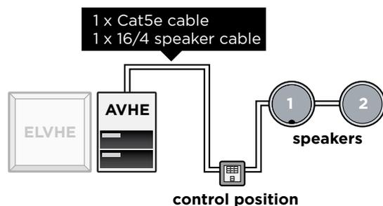
Each audio zone to be wired for multi-room audio will have a Cat5e + 4 core speaker cable run via a suitable control position (typically a switch level backbox), and then from the control position to the first speaker and then looped to the second speaker. This is the principle of the CEA/CEDIA 2030-A standard. Wiring in this way allows for the following options:
