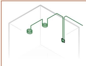
1.5m cable coils should be left at speaker pre-wire locations and 15cm coils in backboxes. All speaker locations should be accurately recorded for future installation.
