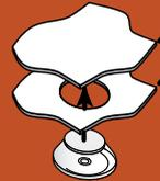
Minimum 200mm diameter void, 100mm clear depth required for installation of in-ceiling speakers
