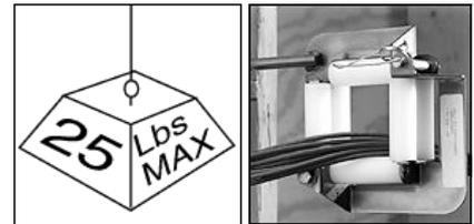
Use a cable pulling accessory. Pull cable using less than 25 pounds (11.3 kg) of pull-force.
