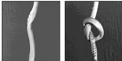
Don't allow the cable to kink, knot or snag while pulling it off the spool or out of the box; deforming the pair-twist will alter the performance of the cable.
