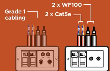
Additional cabling (2 x Cat5e + 2 x WF100) is required for the REMOTE AVHE. Grade 1 cabling (2 x Cat5e + 2 x WF100) should also be available here.
